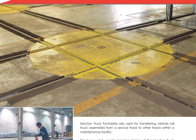
The heavy duty center bearing design of the Macton Truck Turntable rotates the truck assemblies smoothly and provides an extended wear life over turntables that utilize a track and
